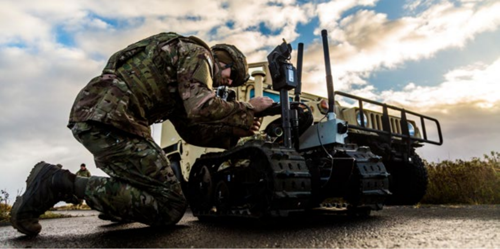
Photo: A US Air Force Explosive Ordnance Disposal (EOD) technician prepares a Mk. II Talon bomb disposal robot for work during exercise Northern Challenge. Credit: NATO
